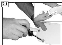
Place blade holders onto blades aligning holes in blade holder with holes in blade. Make sure that the side of the blade you select is facing downward. Install 3 screws and fiber washers to back side of blade as shown. Tighten screws securely. Repeat this process 4 more times until all blades are assembled.
